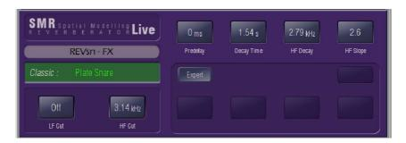
**Spatial Modelling Reverberator**. These provide high quality stereo reverb effects based around 4 complex spatial models - Classic, Hall, Room and EMT. Each of these models employs different reflection and decay algorithms to provide natural sound spaces.
